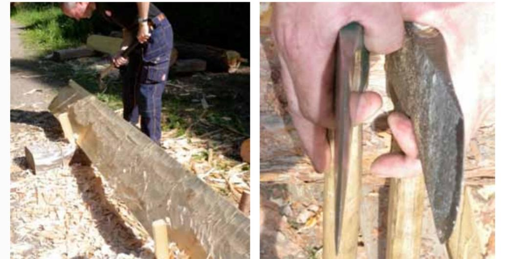
Left: Hewing wood using an axe was the method of creating a smooth surface finish before hand planes were invented in the 12th century. This process is labour intensive, but produces a durable finish as the split face retains closed cells on the surface. Right: The axes used in the workshop demonstration were modelled on traditional axes. Blades of different shapes and weights were made for different purposes.
