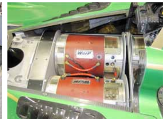
The 'heart' of the green prix machine is the electric motor (red). There are two electric motors in this machine.
