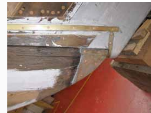
The bottom of the rudder post showing the original copper sheathing, new copper roves and new brass strengthening strips. Also note the new rudder timbers alongside the original.
