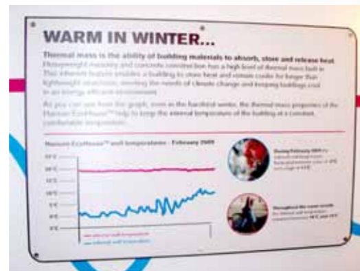
Figure 25: Diagram showing the theory supporting the thermal mass concept.
