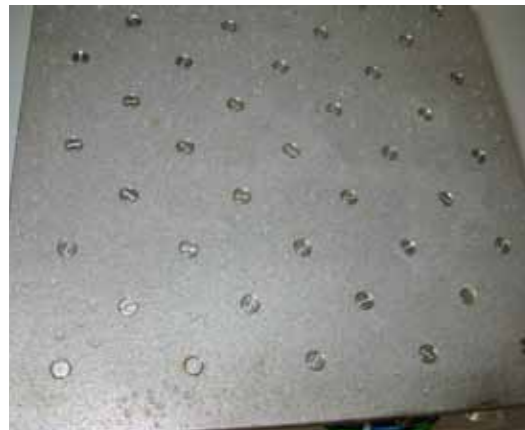
A close-up of the permeable membrane on sweating guarded hotplate at Hohenstein Institute. Image courtesy of the Fellow.
