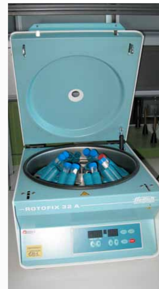
Hydro-extraction of test samples at Centro Tessile Cottoniero. Image courtesy of the Fellow.
