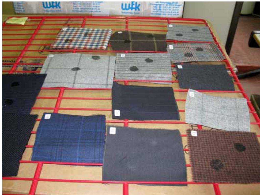
Water spotting test conducted at AWI. Image courtesy of the Fellow.
