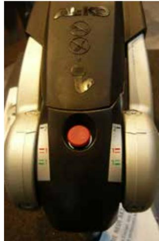
Caravan mounted tow couplings is another area of best practice on display at Dusseldorf. Tow couplings now offer a 'ball load' indicator, which assists the end user when loading the RV prior to departure. This colour coded visual indicator shows when the coupling is correctly engaged.
