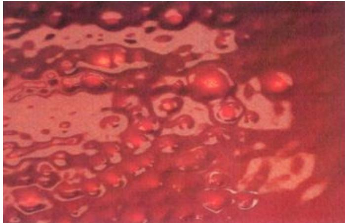
The presence of silicone or oil on the surface does not allow the undercoat or the finish to spread evenly and creates a crater.
