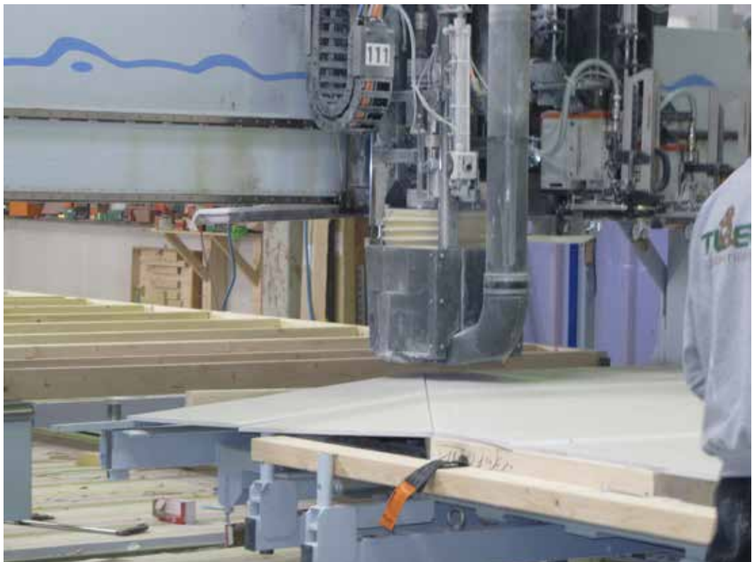
Image: Weinmann machine cutting excess internal lining.
