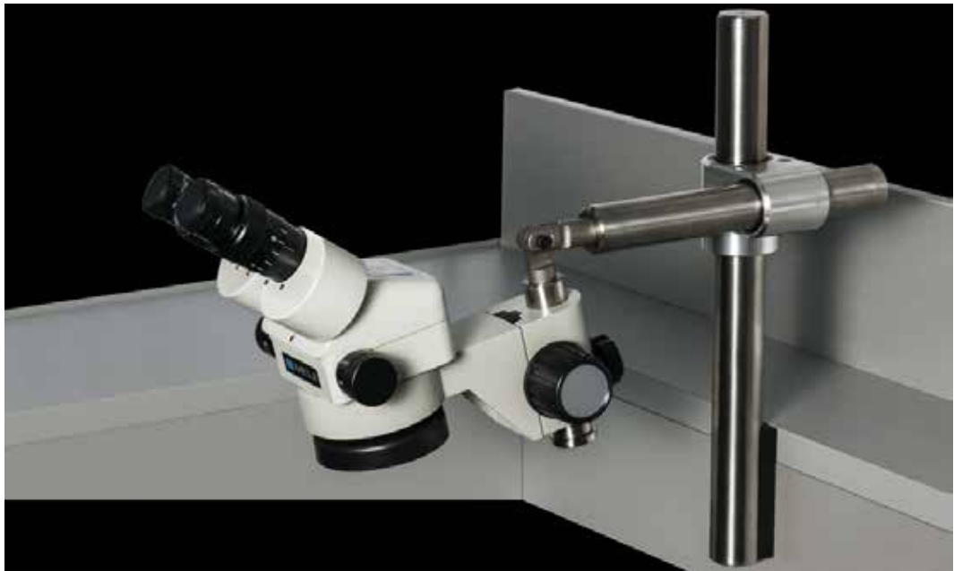
Figure 2. A Meiji EMZ-10 set up with 10 x eye pieces LED ring light and JURA's microscope stand ( www.juratools.com )
