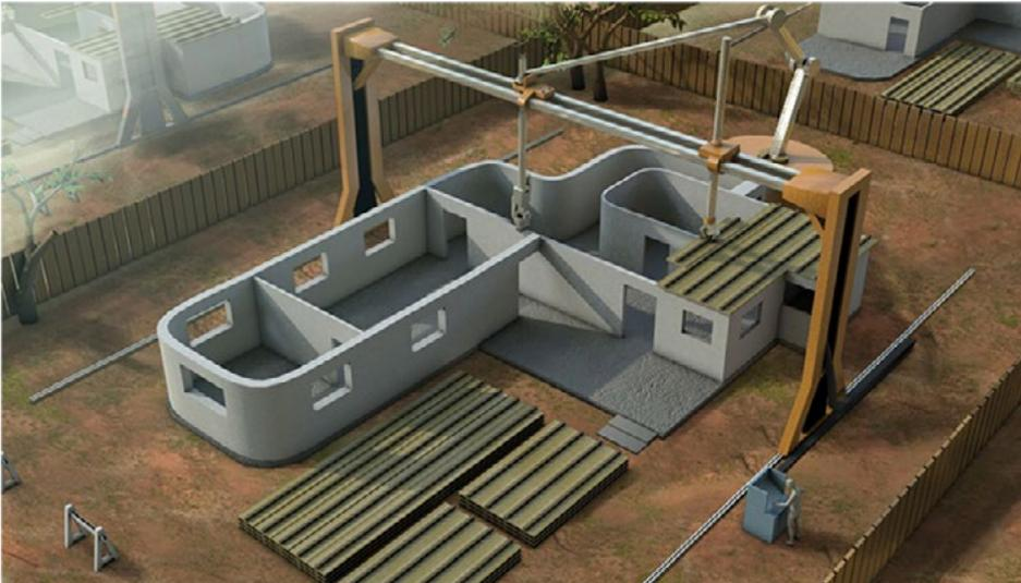
Image 3: A demonstration model for Contour Crafting (Contour Crafting, 2017)
