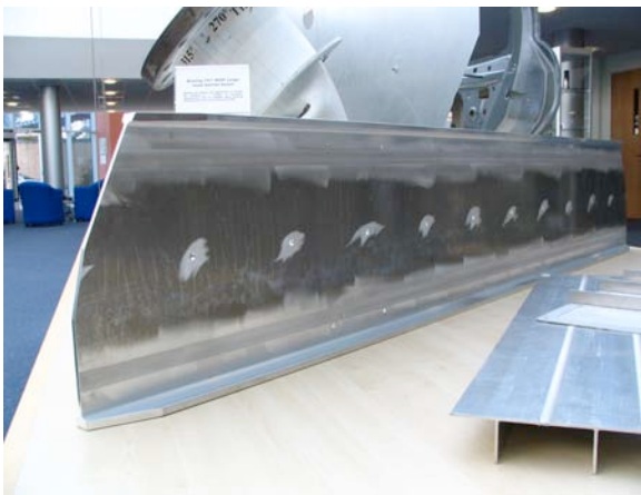
Friction Stir welded components
