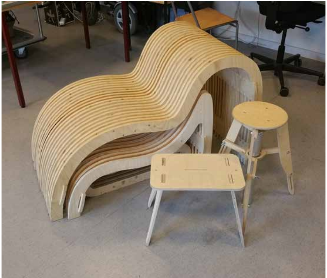
CNC fabricated seats, Fab Lab RUC
