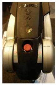
Caravan mounted tow couplings is another area of best practice on display at Dusseldorf. Tow couplings now offer a 'ball load' indicator, which assists the end user when loading the RV prior to departure. This colour coded visual indicator shows when the coupling is correctly engaged.
