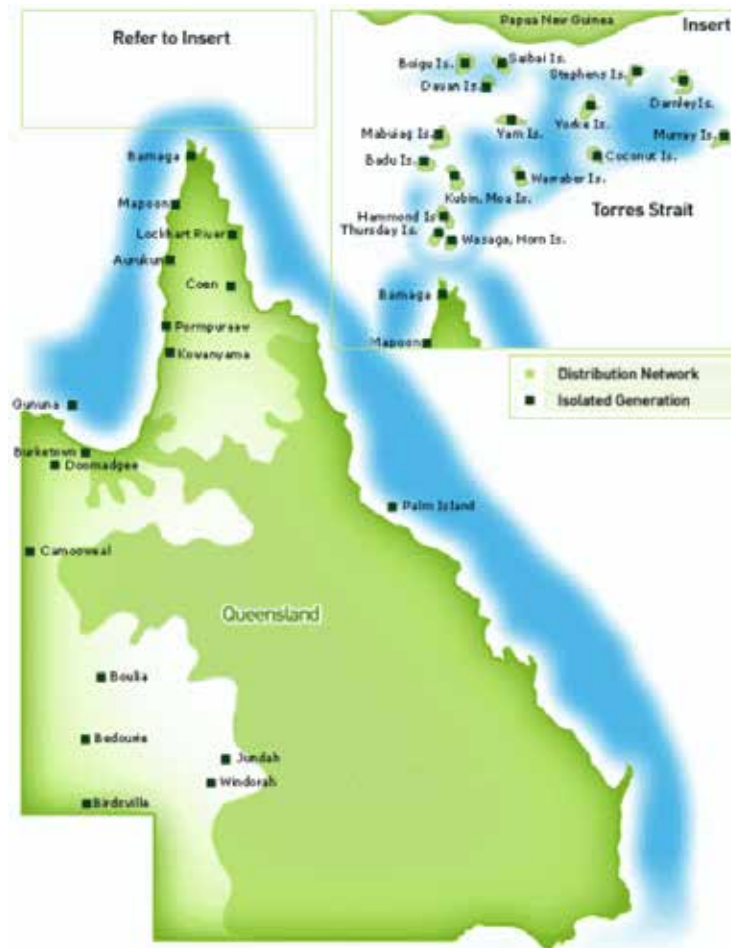
Figure 6. Ergon Energy's power station location map, including 33 isolated power stations that provide electricity to communities which are isolated and too remote for connection to the national grid. 10
