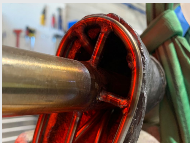
Here you can see the final part of the armature that supports the bottom of the foot. This image demonstrates the extensive work involved in ensuring the sculpture is fully supported, with as many contact points as possible, to provide structural integrity and prevent further damage in the future.
