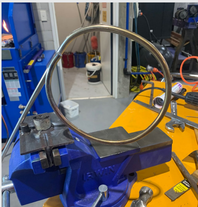
This photo shows Keir bending and shaping one of many rings that would be used to form the armature, providing internal support to the sculpture, using design principles learned from Rupert.
