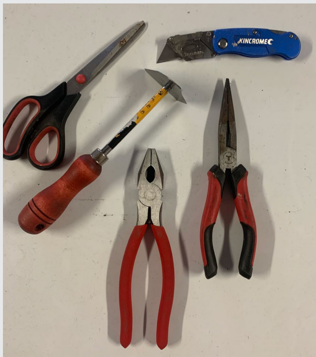
Pliers, lead scraper, scissors and a sharp knife are required for both reshaping and preparation of weld joints
