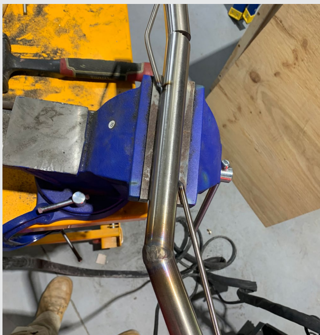
This image shows the formation of one of the main structural bars, which extends from beneath the base of the foot up into the body of the sculpture for added support.
