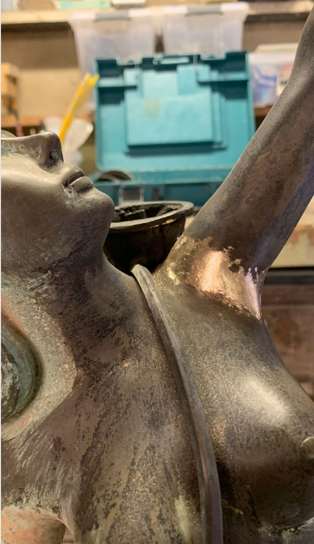
This image shows Keir carefully chasing and finishing the repair to ensure the texture and form of the welded area match the original sculpture.
