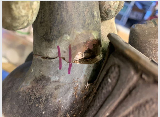
This image shows the arm being carefully aligned with the main body of the sculpture before welding.
