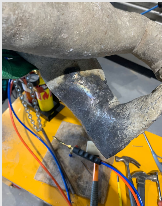
In this image, the foot is fitted and welded to the main part of the sculpture, after carefully adjusting and shaping it with hammers to ensure correct alignment.
