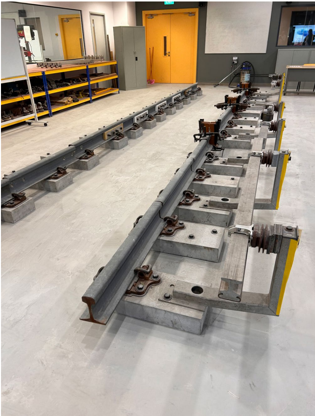
Figure 3. MRT track sections, in engineering workshop at the ITE West, Singapore. Students are trained in Thermite welding.
