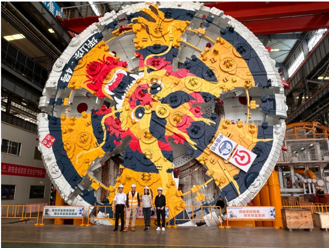
Figure 6. The Fellow standing in front of 14.43 metre diameter cutterhead at the CREC TBM factory, Foshan, Guangdong, with Scott Ma (CREC), Chuyin Zhong (interpreter) and Yan Lee (interpreter),
