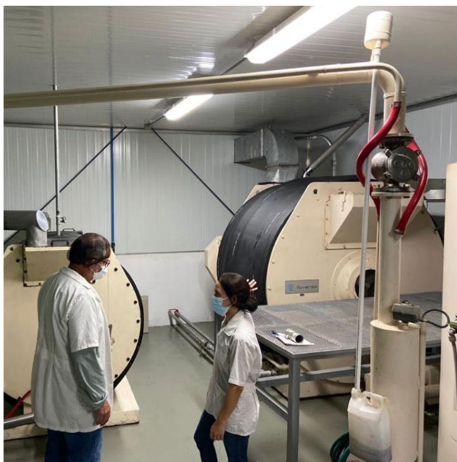
Figure 32. Two of Caribe's chocolate refiners (Photo courtesy of Ecole Chocolat)
