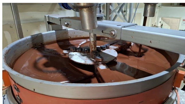
Figure 52. This sieve is 1 metre in diameter, has three arms with brushes that slowly rotate allowing the chocolate to pass through and catch any foreign objects. It also vibrates assisting the chocolate to pass through.
