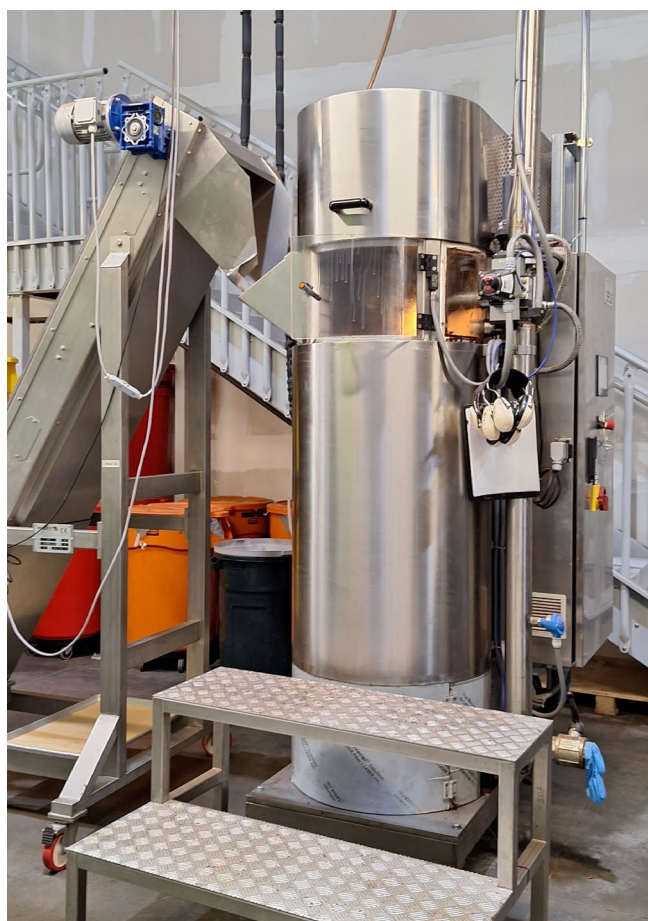
Figure 50. First ball mill where the pre-ground beans are refined into cocoa liquor / cocoa mass
