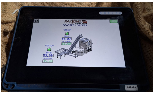
Figure 46. Each piece of equipment in the production line is controlled on an iPad (stop, start, temperature, time volume etc)
