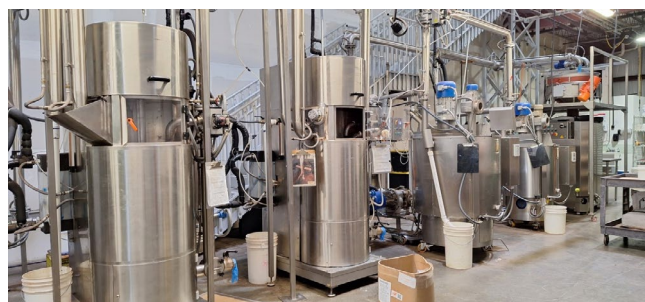
Figure 51. Production line - from left to right: two ball refineries, two conches, strainer above the holding tank.
