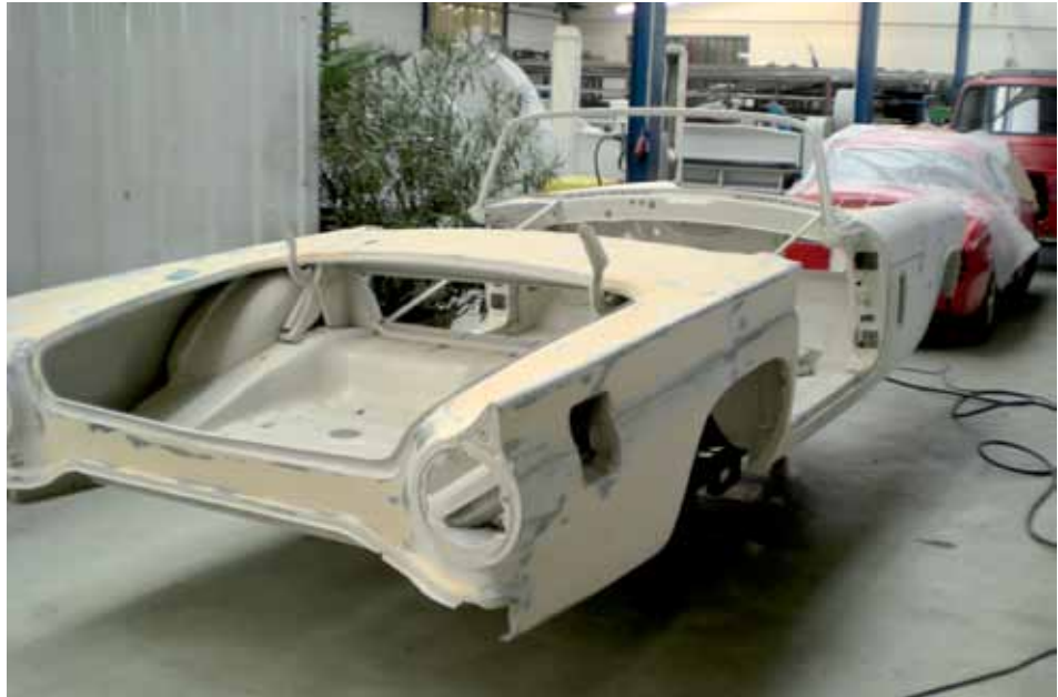
Car repaired using plastic filler at Brixner GmbH, Germany
