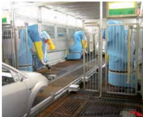
Enamel clear coat robots for door shuts. The robots sleep until the car breaks the infra red beam and then they start application. This saves energy.
