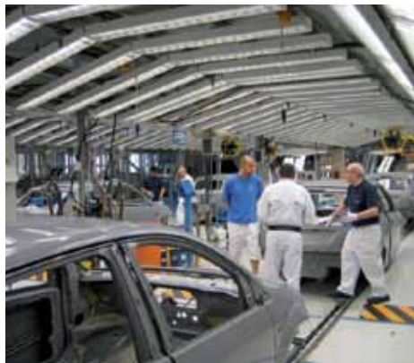
Primer sanding/enamel preparation. There is abundant florescent lighting so that faults can be easily detected.
