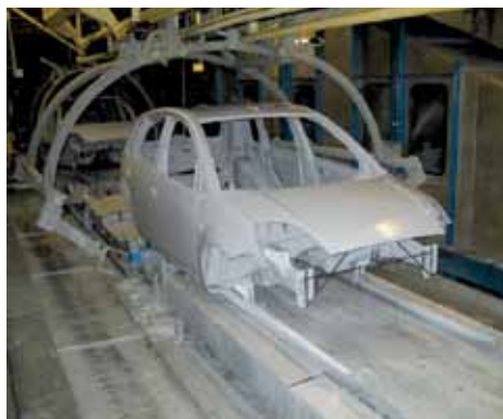
Pre-treatment auto-unload (wet body before oven)
