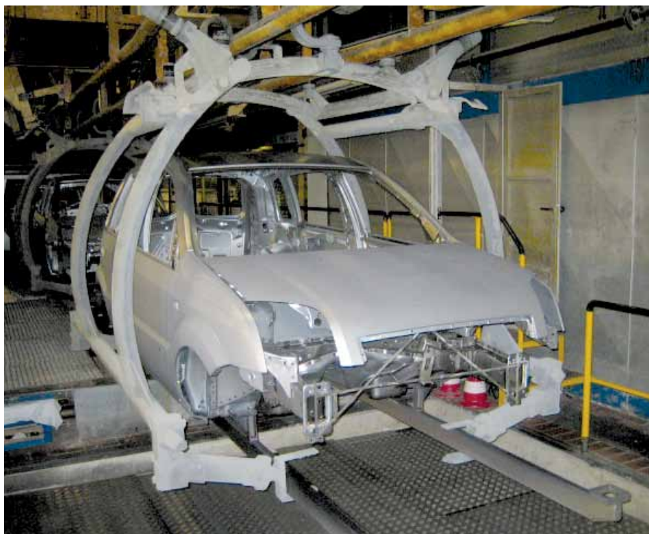
Pre-treatment entry. This is the beginning of the paint production line. Prior to this stage the car is checked for dents, scratches and marks. Anything found is rectified before entering the pre-treatment area.
