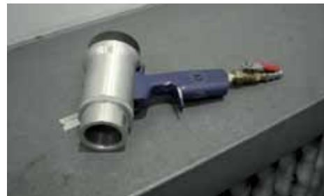
Hand held dryer with interior filters in order to reduce the chance of dust being blown onto the paint work
