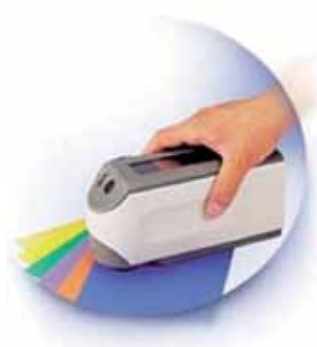
A spectrophotometer measures colour and generates numerical data for analysis.
