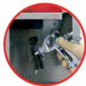
Flushing and cleaning the paint channel and air cap, approximately 21 seconds.
