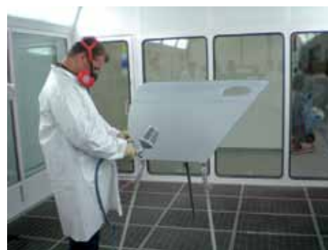
Step 2 – application of water-based primer at SATA training centre
