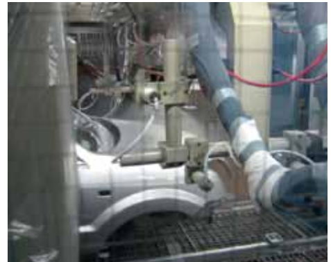
Enamel Clear coat applied by an ESTA machine (robot)
