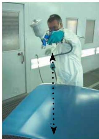
50-60cm distance for drop coat application
