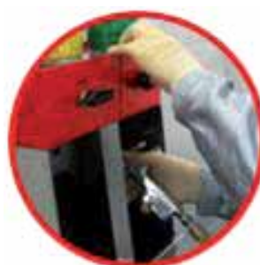
Dry blowing; used cleaning liquid is collected. Approximately four seconds.
