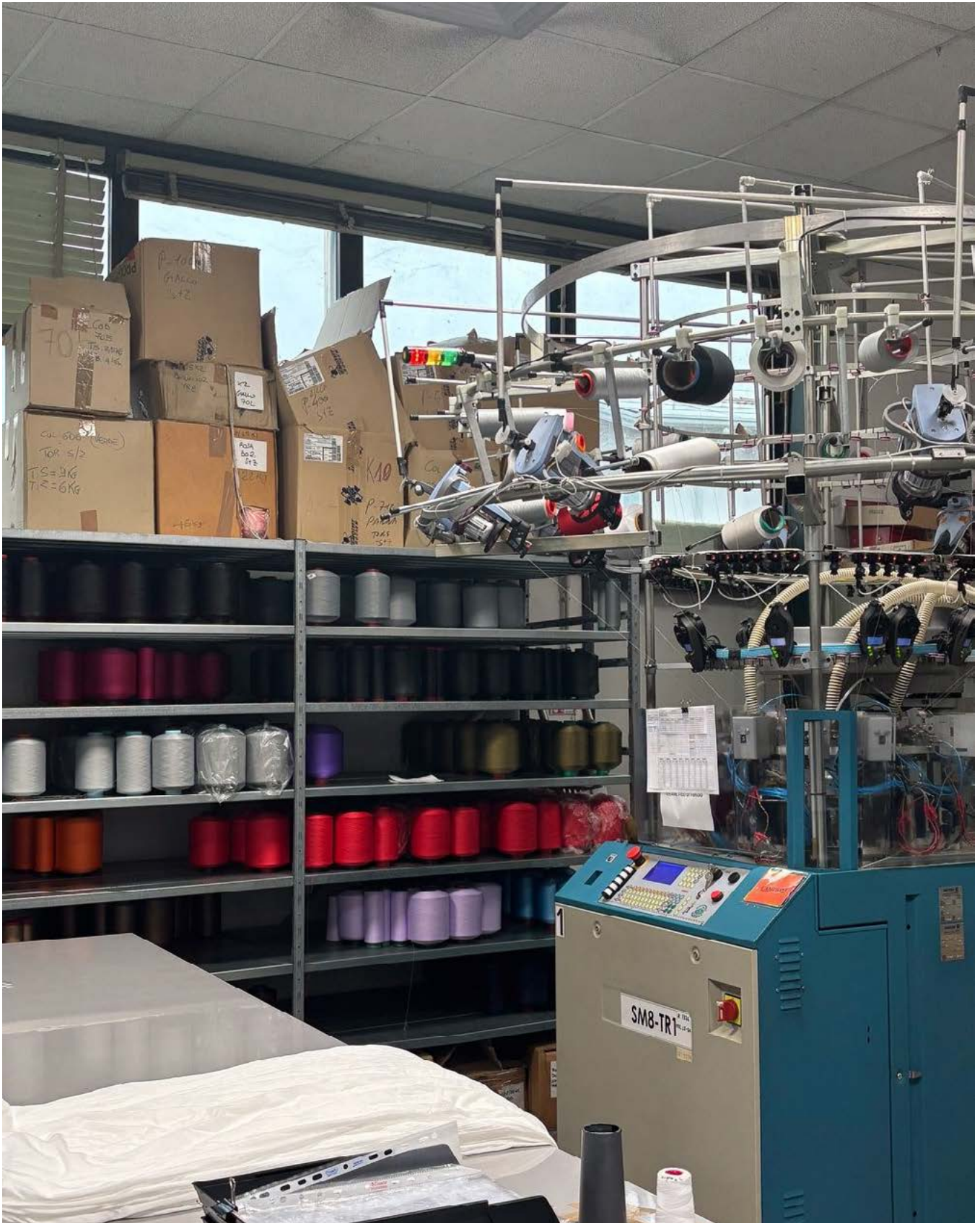
Figure 4. Production facility floor showing circular knitting machines and yarn creel systems — Nesatex, Carpi. This facility was the primary site for hands-on sampling during the Fellowship.
