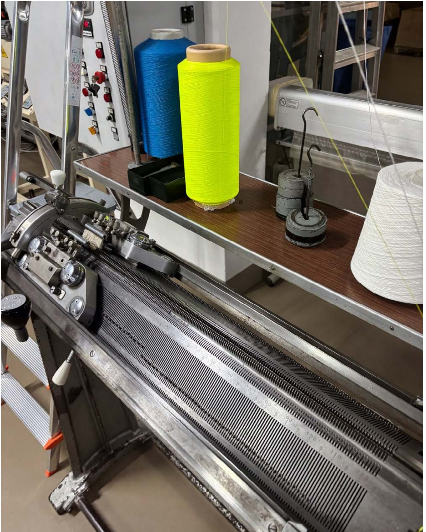
Figure 9. Flat knitting machine needle bed with yarn cones — the individually controllable needles visible across the full width of the bed, enabling zoned stitch structures within a single panel.
