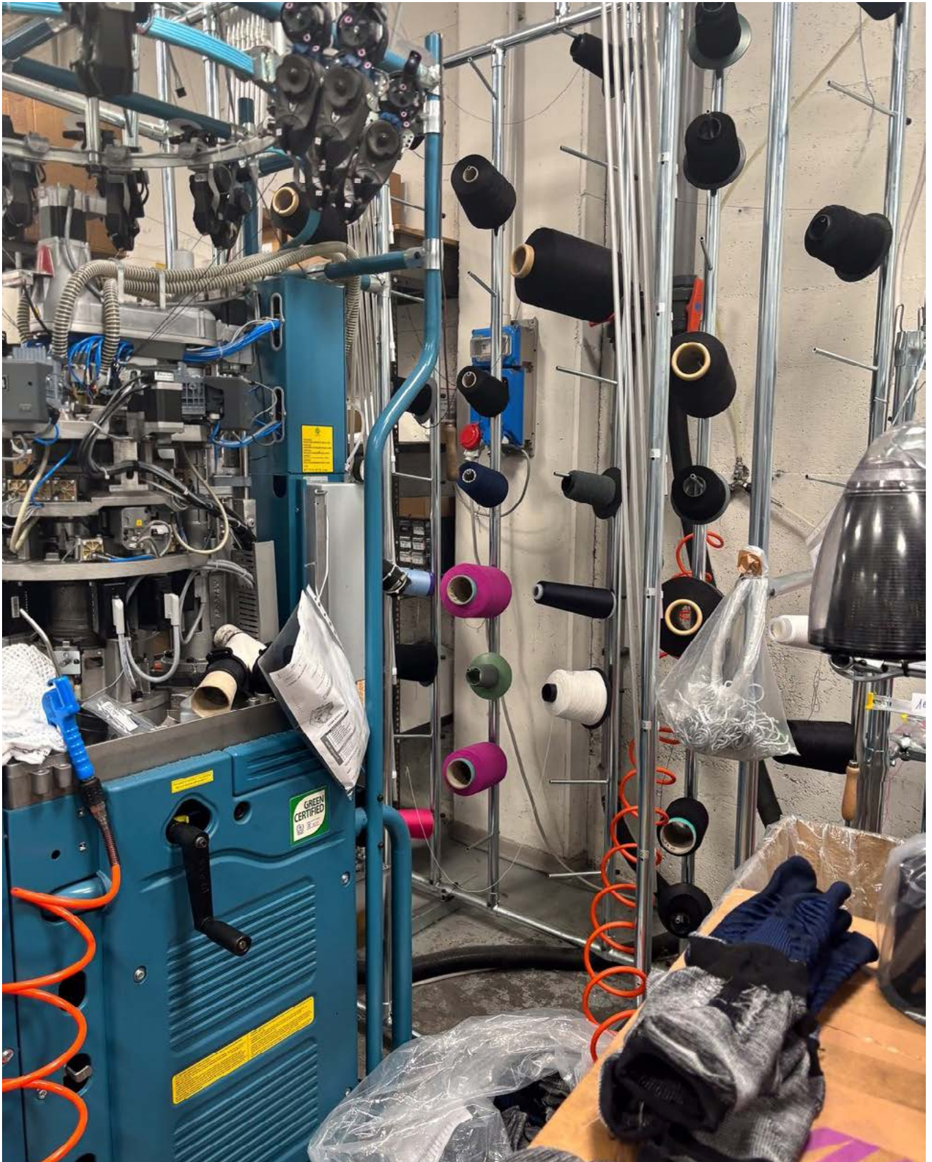
Figure 2. Circular knitting machine close-up showing yarn creel feed system — each of the 48+ cones feeds a separate yarn carrier, illustrating the scale of yarn commitment required for a single circular production run.
