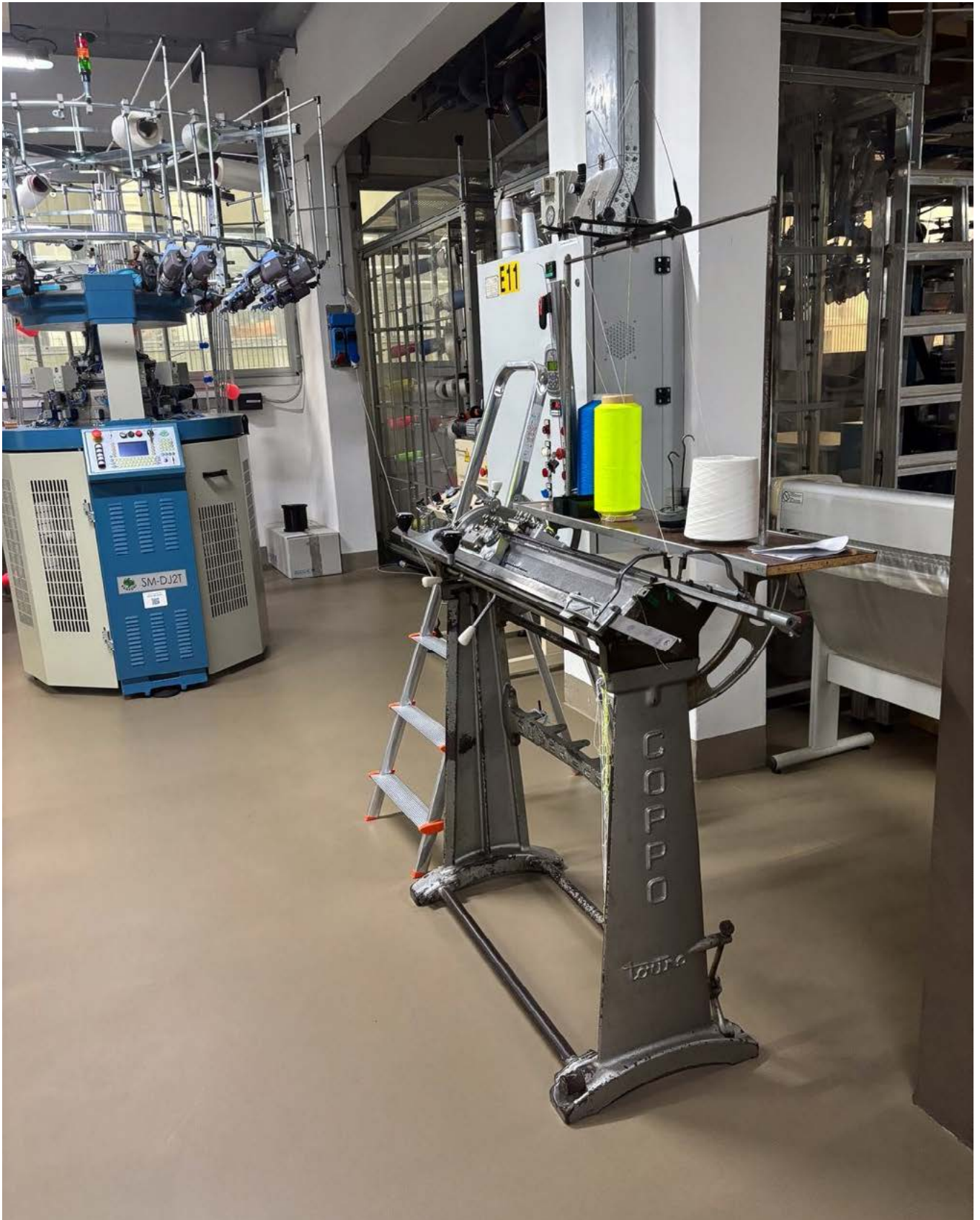
Figure 10. Heritage Coppo flat knitting machine alongside a modern Santoni circular machine — the coexistence of traditional and advanced technology in Italian facilities illustrates the depth of accumulated knowledge that informs contemporary practice.
