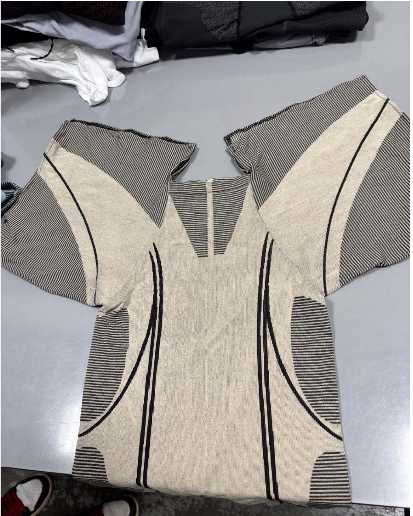
Figure 6. 3D engineered knit panel laid flat — illustrating zoned stitch architecture with distinct structural, mesh, and patterned areas mapped to functional zones of a garment or furniture cover.
