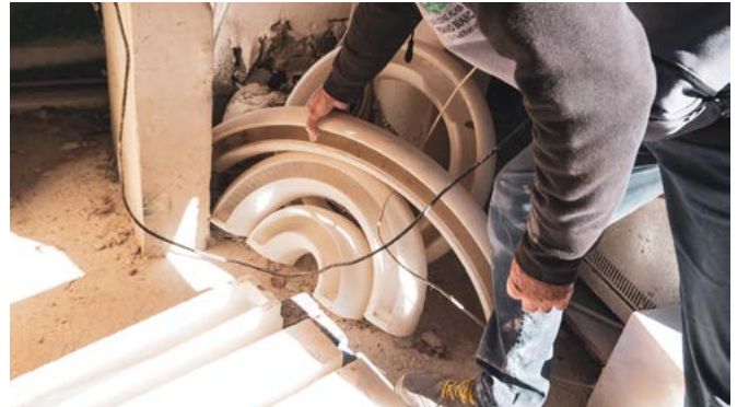
Figure 40. CNC-cut alabaster lighting components before hand finishing. Image credit: Marlo Lyda.
