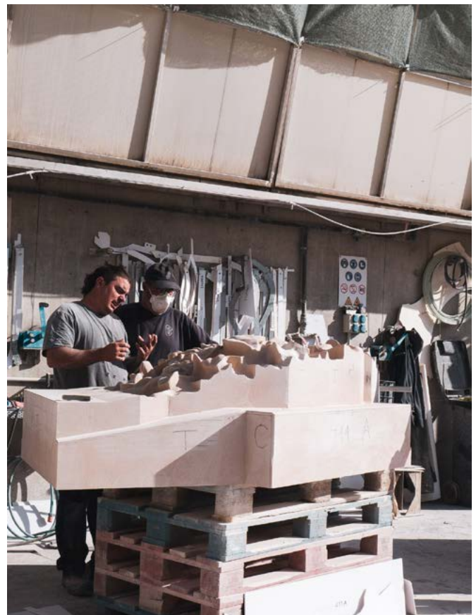
Figure 24. Craftspeople discussing hand finishing for a Sagrada Família façade, with reference templates in view at Barbany Artesans. Image credit: Marlo Lyda.
