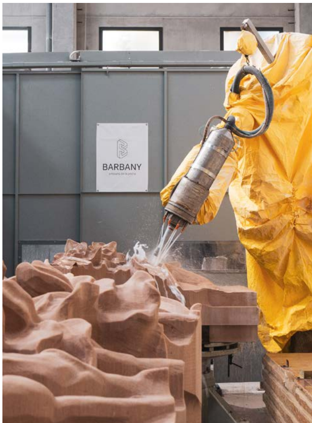
Figure 23. Sagrada Família façade component being CNC-machined at Barbany Artesans. Image credit: Marlo Lyda.
