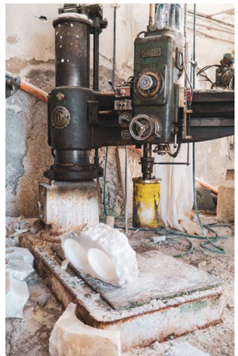
Figure 35. Industrial hole-saw drill used to cut alabaster blanks for turning and handwork. Image credit: Marlo Lyda.
