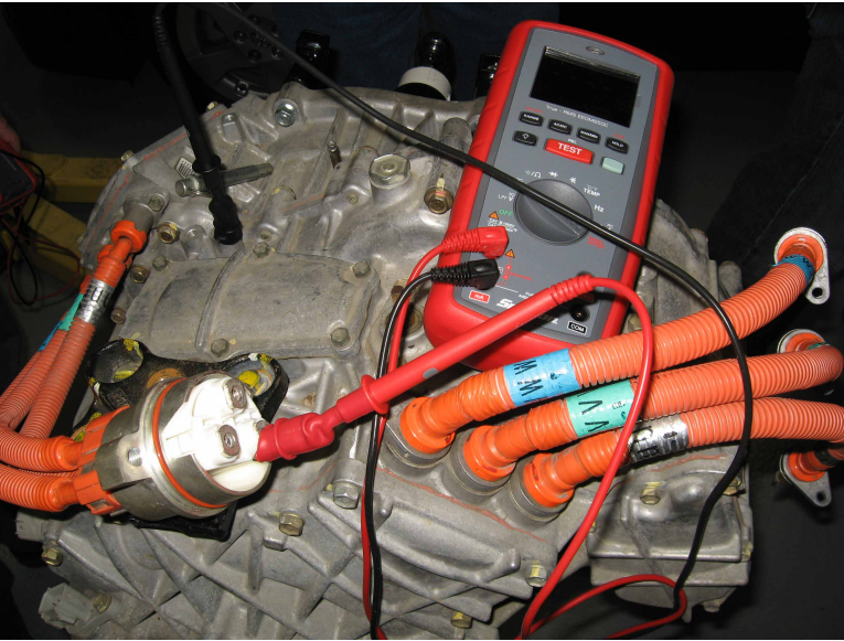
Left: Prius high voltage wiring being tested with a megaohmmeter. Note the orange conduit.
