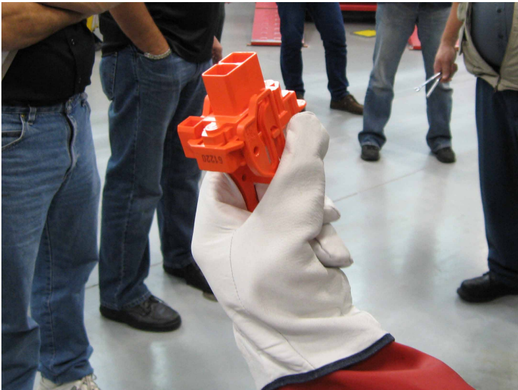
Above: Removed Prius service plug. Note the use of approved linesman’s gloves and with leather over-gloves.
