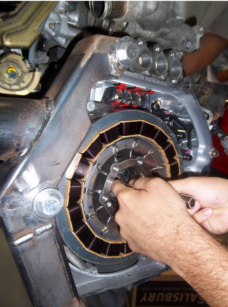
Above: IMA windings on the rear of the ICE. The rotor is being fitted with the special tool for removal.
