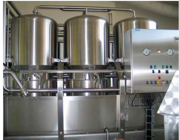
Overhead tanks used to distribute the curds evenly between the six moulds.
