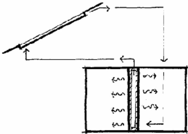
Fan assisted air into the edge of the slab
