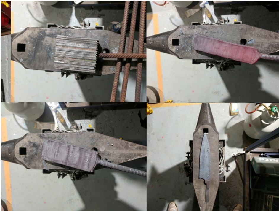
A Pattern Welded Blade or "Damascus" blade being made.
