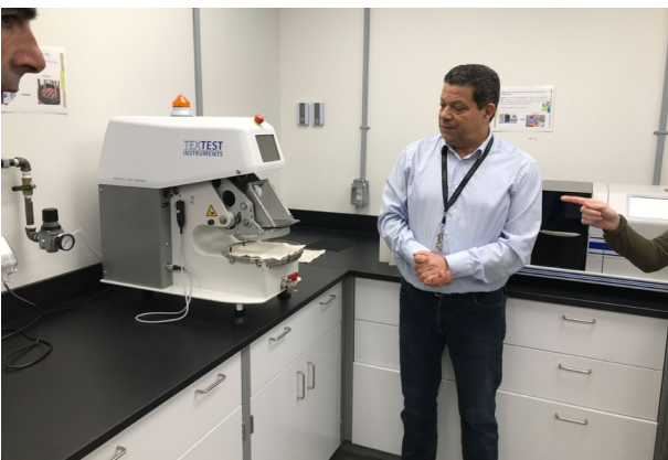
Figure 72. Vestechpro Materials wind permeability testing machine
