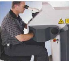
Focusing the Microscope (image courtesy of Rofin Laser Micro)
