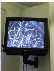
Monitor for training purposes. A camera is fitted to the microscope to enable the image, seen by the operator, to be viewed on the monitor by trainees (image courtesy of The Fellow)
