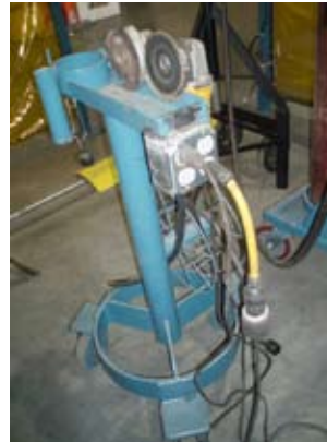
Pipe Fitter's portable power tool stand
