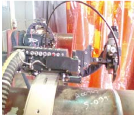
Liburdi orbital welding machine, UA Instructor Training Program Ann Arbor 2006
