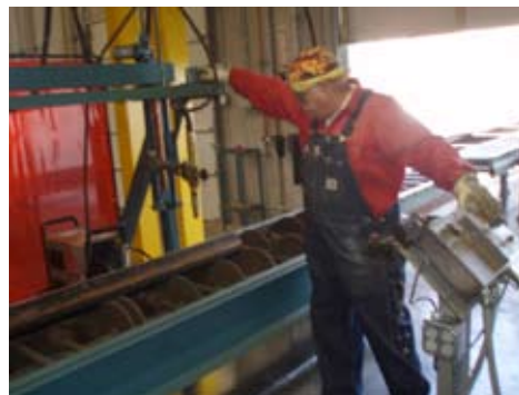
Pipe fitter demonstrating plasma cutting machine cutting pipe at the Southland Industries.
