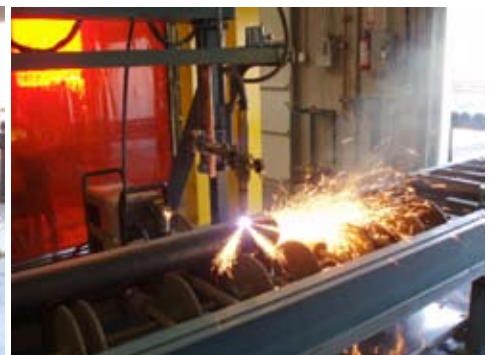
Pipe fitter demonstrating plasma cutting machine cutting pipe at the Southland Industries.
