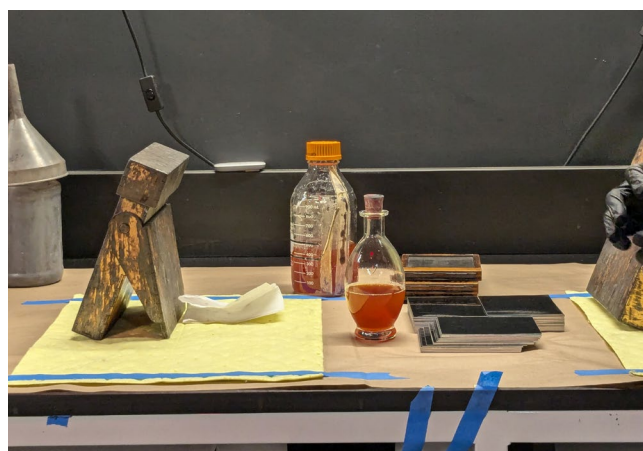
Figure 6. Set up for coating a plate with collodion and sensitising it with silver salts
