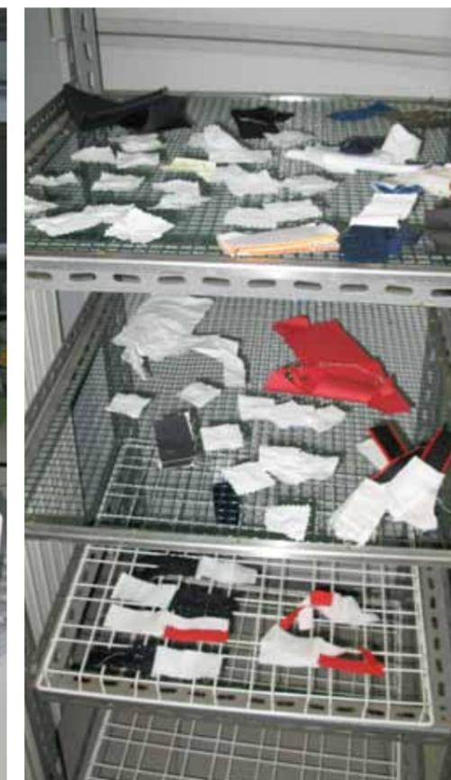
*Colourfastness test specimens drying at Centro Tessile Cottoniero. Image courtesy of the Fellow.*
