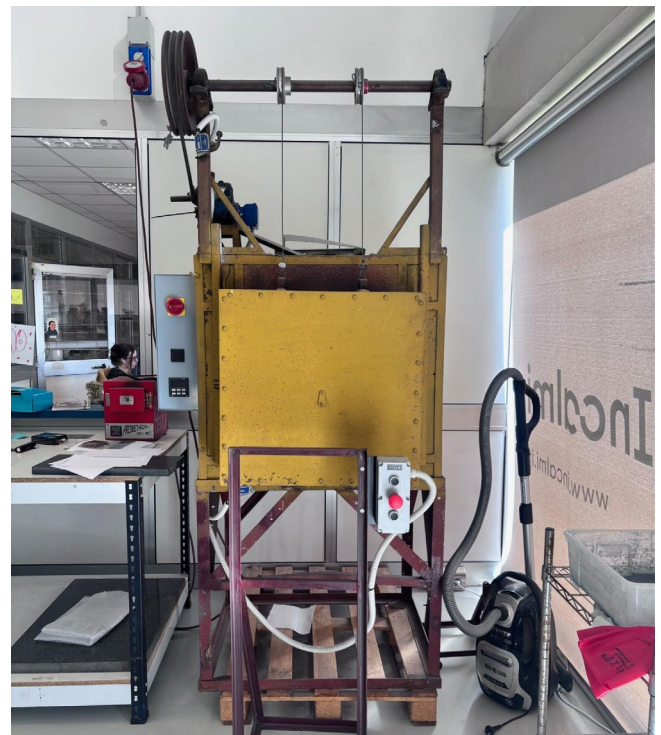
Figure 25. The original kiln Incalmi used when first learning vitreous enamelling, Marghera.
