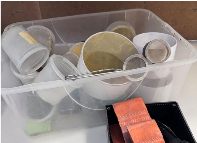
Figure 32. The enamelling workbench at Incalmi, with the simple mesh tools used to apply enamel powder.
