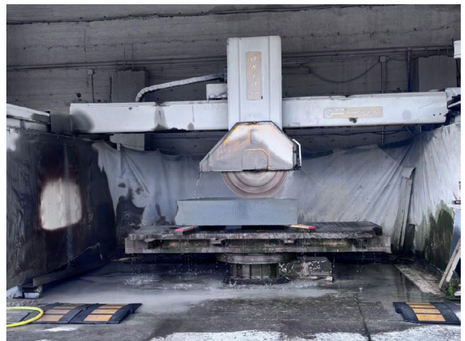
Figure 53. A raw lava stone block being wet-sawn into slab format.
