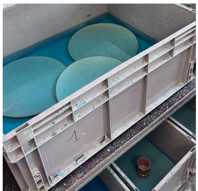
Figure 28. Copper tabletop substrate in the pickle solution, removing firescale and oxides before degreasing and enamelling.
