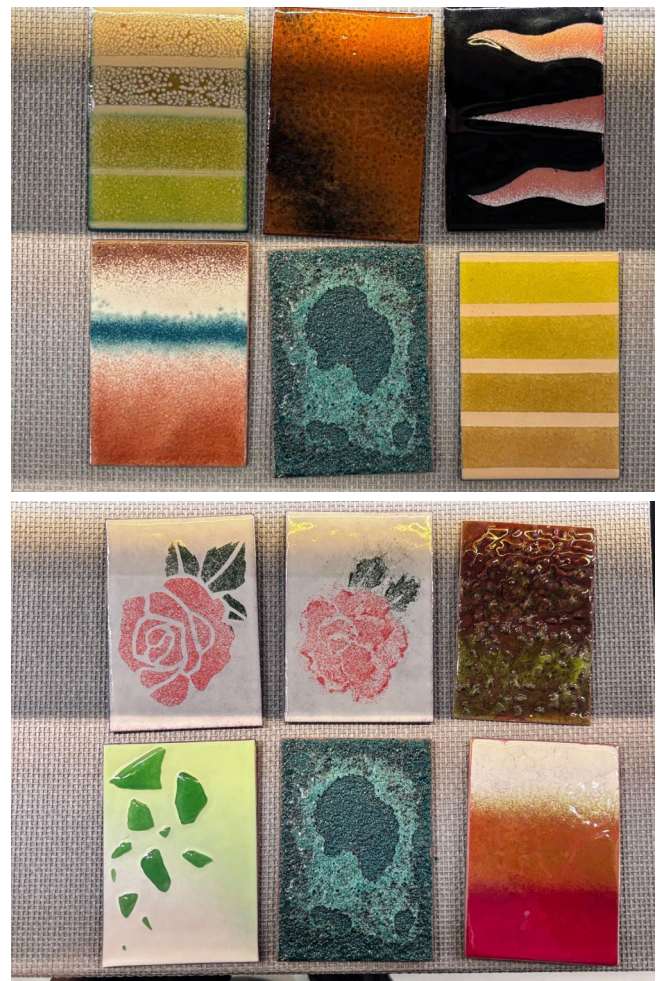
Figure 23. Pattern, colour and texture enamel tests, developed for designer collaborations including Valentina Cameranesi Sgroi, Incalmi.
