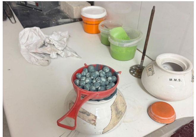
Figure 72. Ceramic balls and jars used to grind flux and pigment into liquid enamel.
