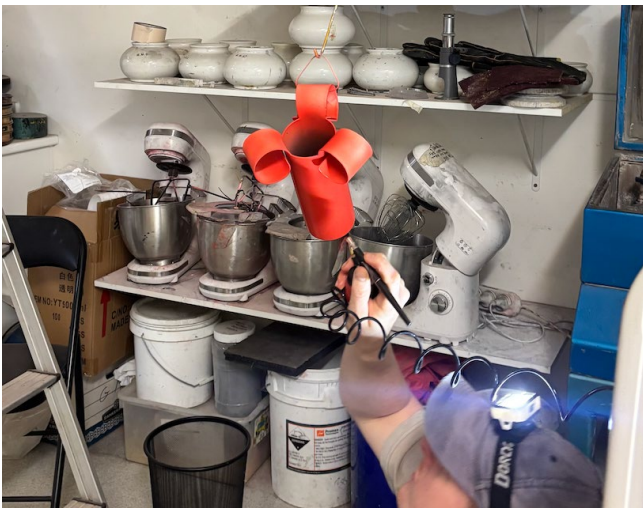
Figure 75. Enamora vase, Set up small air brush gun (purchased specifically for the project) to test gradients and layering of wet Vitreous Enamel.
