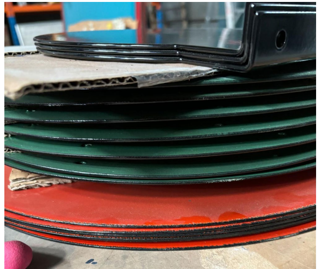
Figure 13. Pre-coated signage in Peter Magalotti's workshop, showing edge burnout, where exposed metal edges re-oxidise during successive kiln firings.
