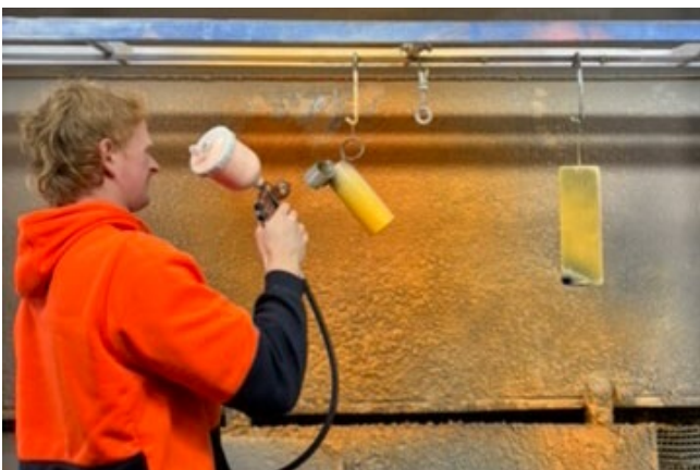
Figure 76. Enamora vase, Testing large spray gun and how we could combine the two application techniques to achieve desired finish.
