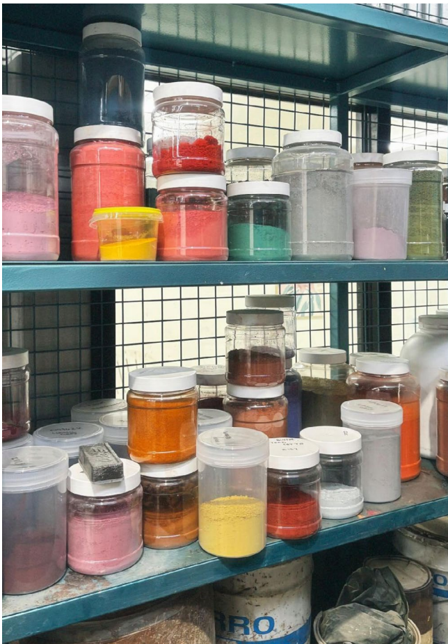
Figure 71. Coloured pigments for the vitreous enamel mix.
