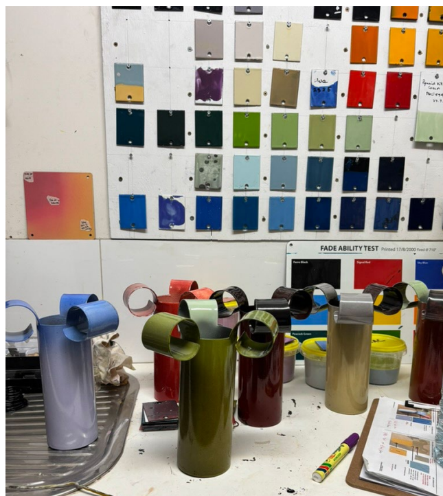
Figure 81. Enamora vases, post firing. Reviewing against colour chips in the factory's lab.
