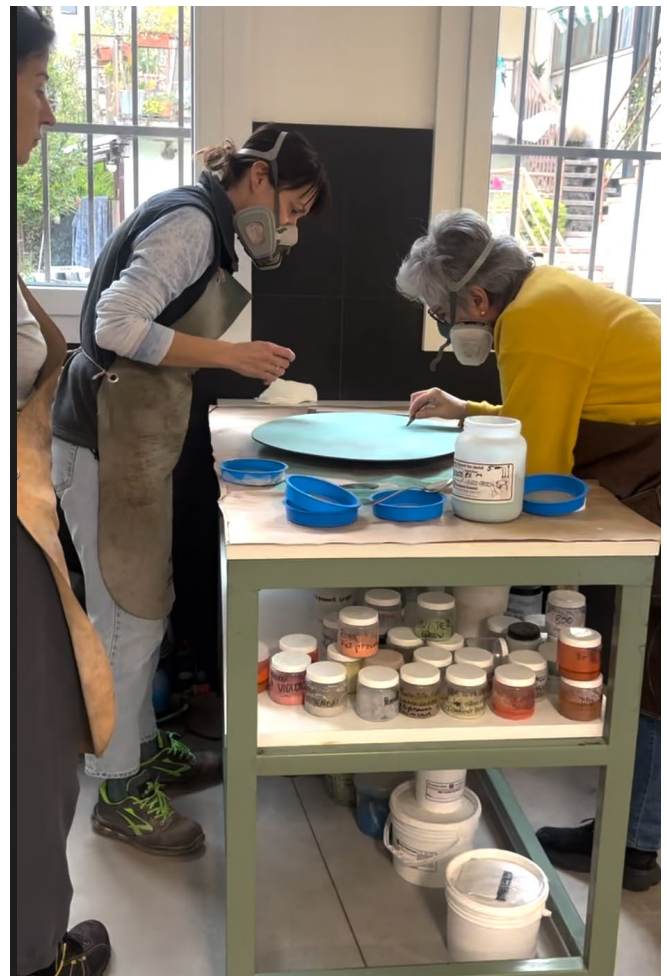
Figure 2. Alessandra Malfatti & assistant Applying powdered enamel for the Paola Lenti table Top designs.
