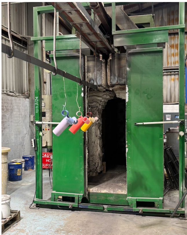
Figure 79. Enamora vase, Entering Kiln for 750 degree celsius firing for 15 minutes.
