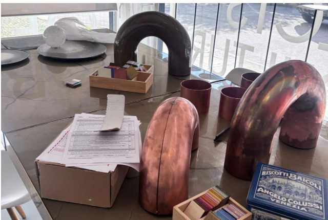
Figure 33. Complex three-dimensional enamelled forms, Incalmi, whose welding required extensive testing before enamelling could begin.
