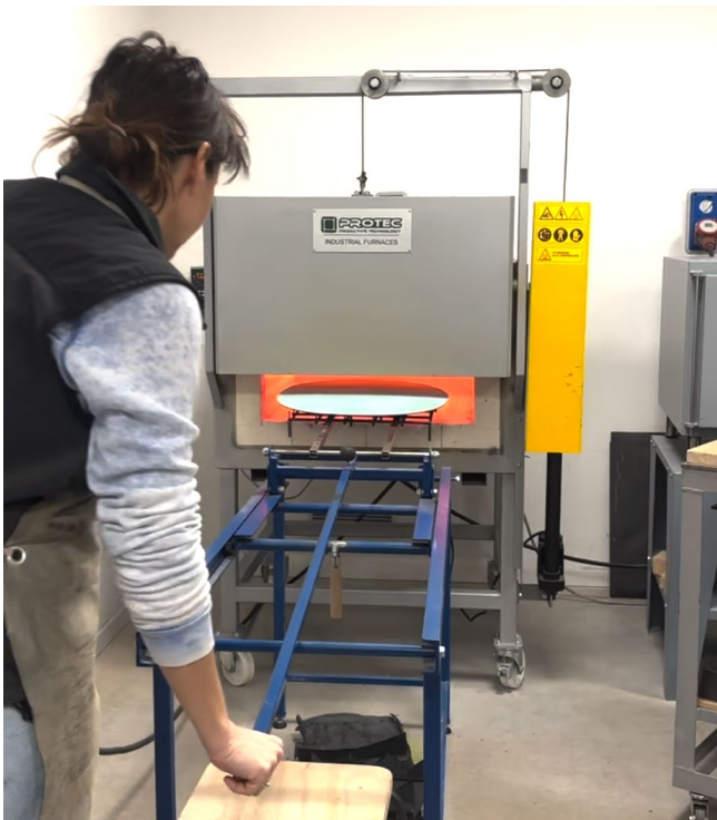
Figure 42. An assistant placing a freshly powdered tabletop into the kiln.
