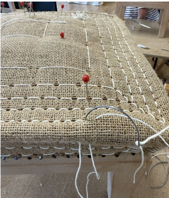
Figure 5. Tabouret carré process – Stitching.
