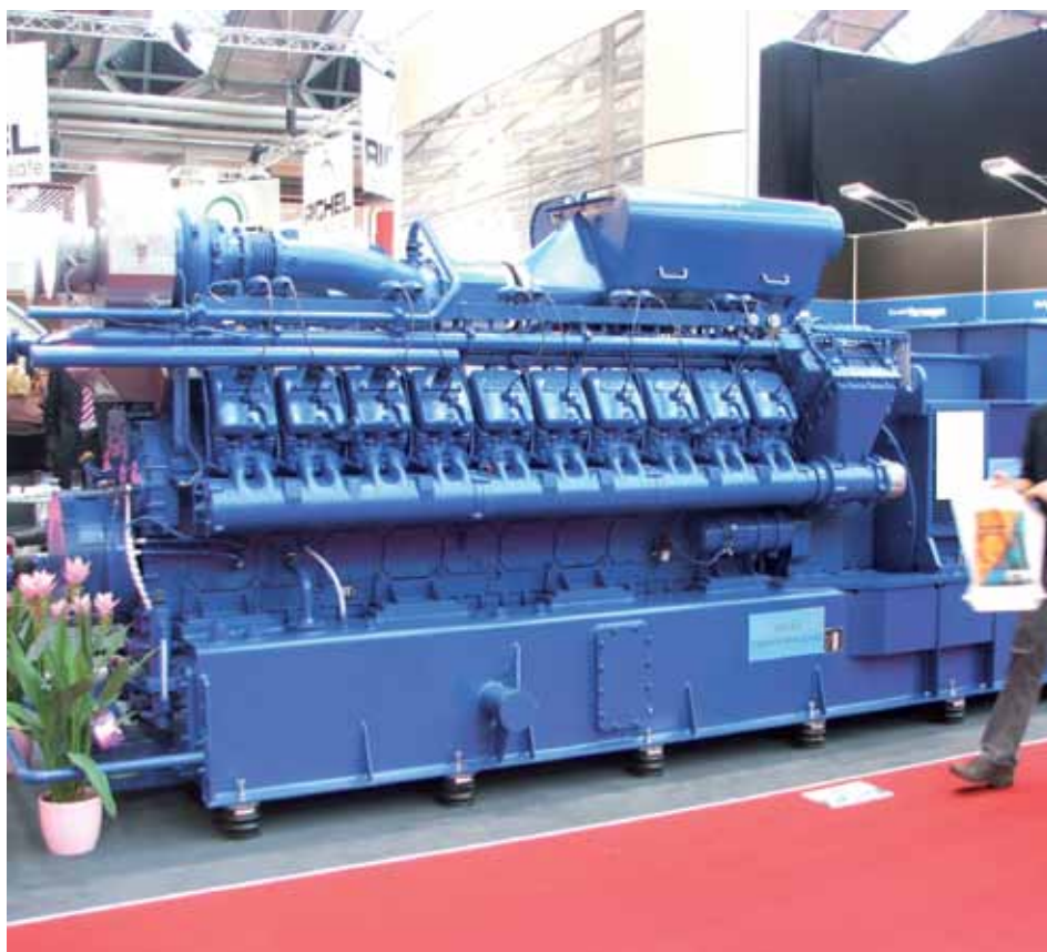
Combined heat and power generation unit at Horti Fair, Amsterdam
