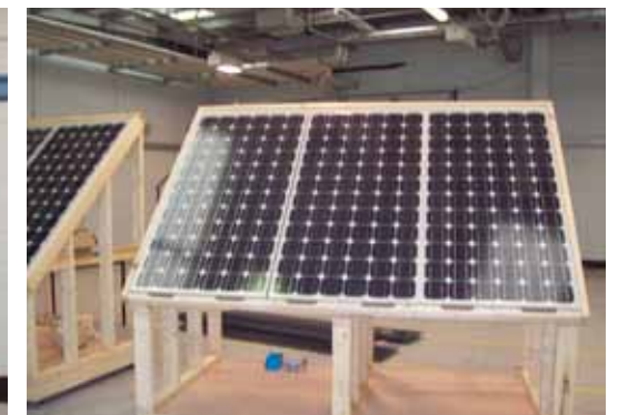
Figure 22: Photoelectric panel system workstation used in electrical training
