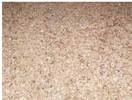
Figure 40: The typical soft wood chips used in the biomass system from local woodland material
