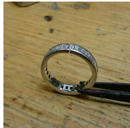
Image 11a and Image 11b: A diamond set platinum ring. The ring is broken right through but soldering would heat the entire piece resulting in damaged diamonds. Image on right shows the weld completed with filler wire building up the join, ready for the finishing process. Because welding made a repair possible, a full remake of the ring has been avoided.
