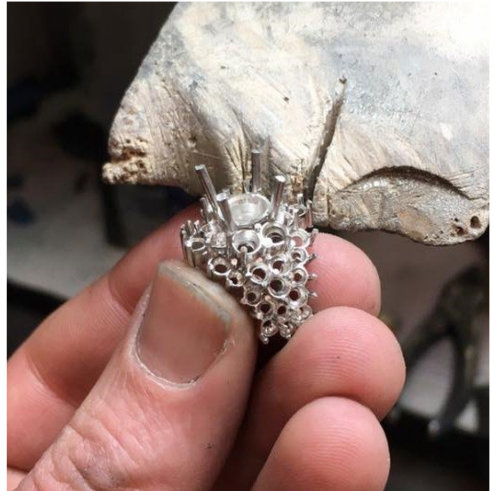
Image 17: A complicated diamond cluster ring being assembled using spot welds to “tack the pieces together”, before final joining later (work and photo courtesy of Harry Rose, jeweller).
