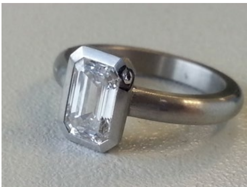
Image 13: The diamond set platinum ring has just been made and the diamond set into it as the last stage of construction. However, a small crack appeared in the corner of the setting which could not be soldered without risking the diamond. The welded repair (shown with permanent marker) within a millimetre of the diamond is a successful save of the entire piece.
