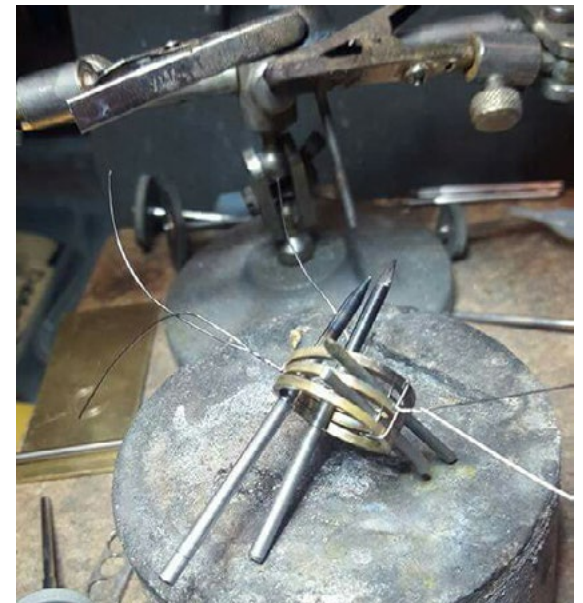
Image 15: A ring comprising three bands being joined together using the soldering technique. Here the jeweller is using complicated arrangement with spacer metal and binding wire holding the shape while the melting temperature is achieved under the torch. (photo courtesy of Young Jewellers Facebook Group)
