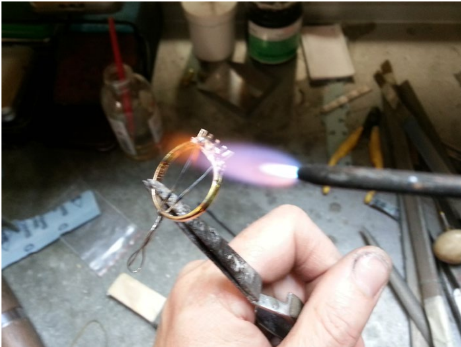
Image 16: An opal ring that is held together with binding wire to enable the setting to be soldered into place.
