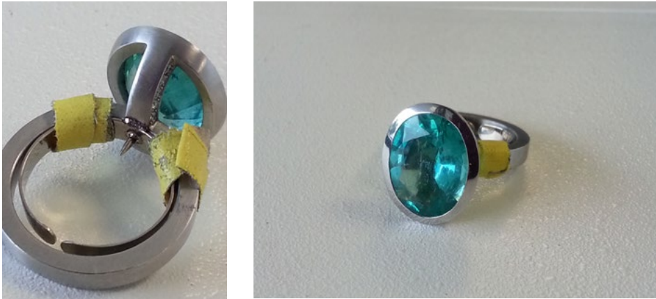
Image 12a and Image 12b: An emerald ring Noble photographed during alteration. A sleeve of springy metal is being added to the inside of the band to make it smaller to fit the wearer. This would be impossible with soldering techniques as emeralds are extremely fragile and heat sensitive. Even removing the emerald from the setting would probably require complete destruction of the ring mount, meaning that remaking would be the traditional solution here. The simple weld behind the setting shown has provided a solution which is vastly less time consuming and costly.
