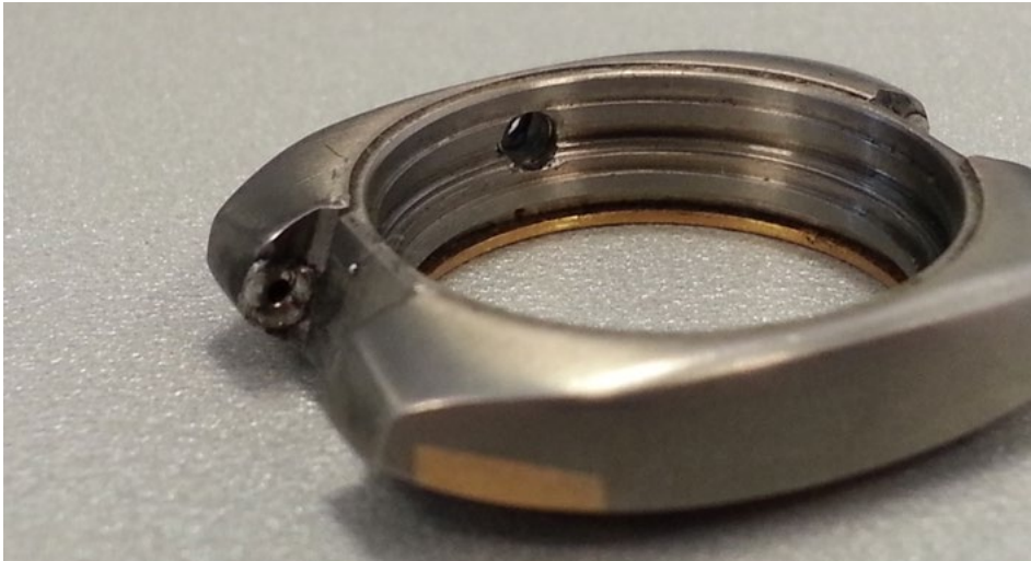
Image 20: Gold and steel combined in a watchcase.
