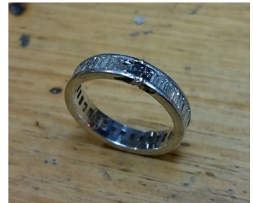
Image 11a and Image 11b: A diamond set platinum ring. The ring is broken right through but soldering would heat the entire piece resulting in damaged diamonds. Image on right shows the weld completed with filler wire building up the join, ready for the finishing process. Because welding made a repair possible, a full remake of the ring has been avoided.
