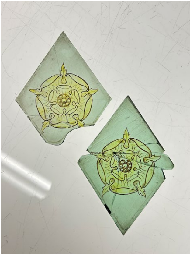
Figure 12. Image one: Edge bonding achieved with CAF 3 silicone at Barley Studios
