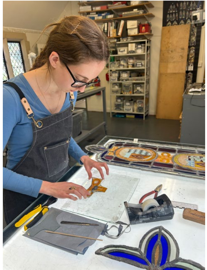
Figure 13. Image two: Edge bonding with Araldite 2020 at York Glaziers Trust, photo courtesy of York Glaziers Trust
