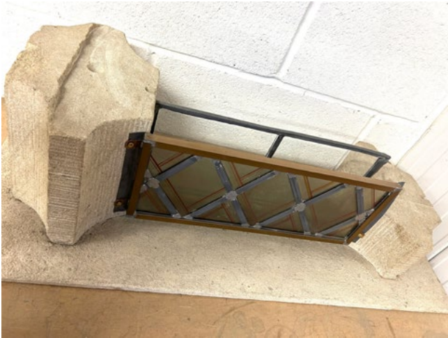
Figure 15. Internally ventilated model: note the framed historic stained glass fixed to the internal masonry, with an external protective glazing panel separated by a ventilated interspace.
