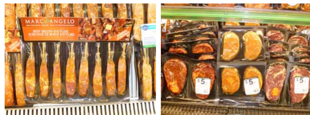
Chicken skewers packaged using VSP (Vacuum Skin Packaging), Walmart Pork and beef steaks packaged using VSP, Walmart
