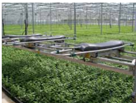
Overhead gantry units
