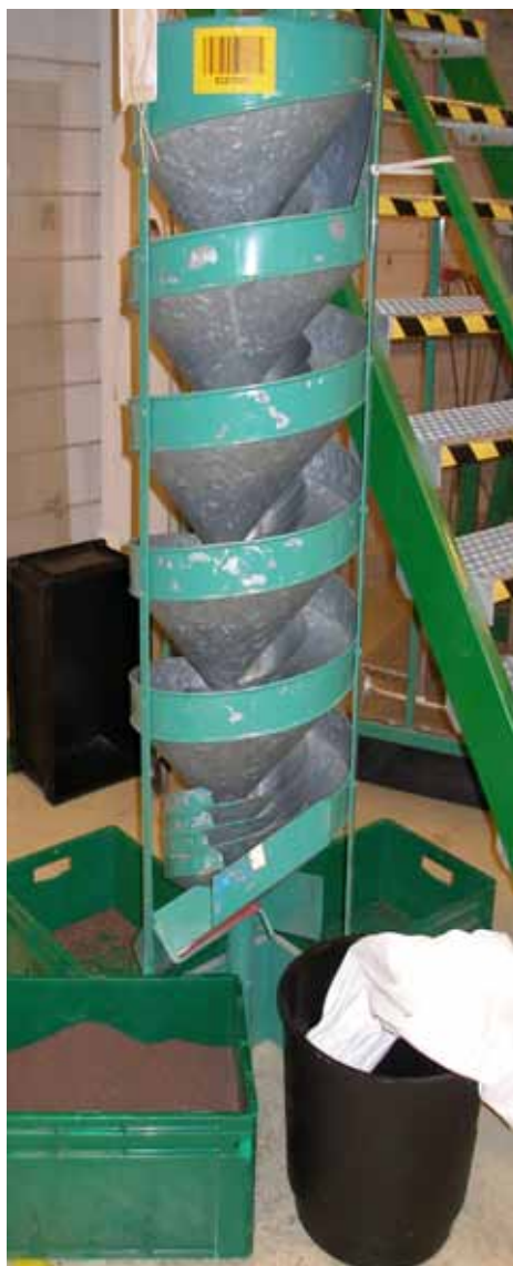
Seed being graded for size
