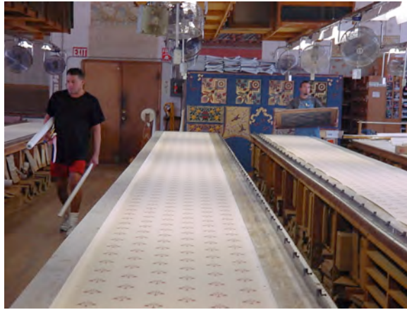
Benches with complete roll ready for printing.
