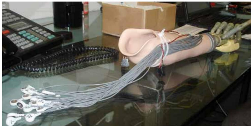
Figure 8: Prosthetic hand with electrodes, showing the various connecting leads from the neuroprosthetic hand to the human brain.
